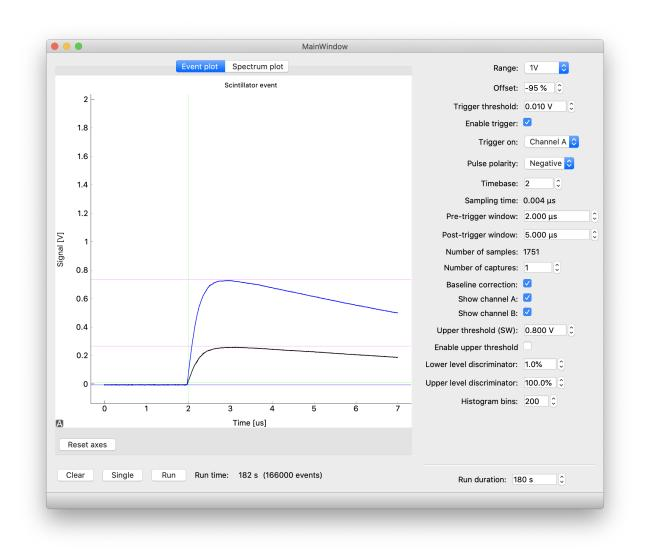
Fig. 2: Screenshot of the GUI showing a plot of a gamma detection from a nuclear source (sodium-22). The green guides show the instant of triggering (vertically) as well as the trigger level (horizontally). The purple guides show the measured pulse height and the blue guide shows the measured baseline.
