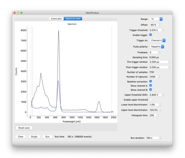
Fig. 1: Screenshot of the GUI showing a plot of the gamma spectrum of a nuclear source (sodium-22, black line). Another detector at the opposite side of the source picks up coincident annihilation radiation gammas.
